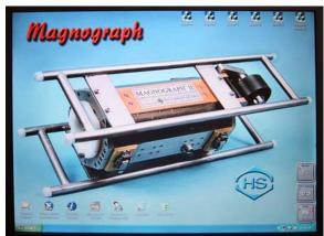
The upper right corner of the Magnograph™ desktop contains separate icons corresponding to five rope size ranges and another icon for the playback of data. A left click on any of these icons starts the MagWin software.
